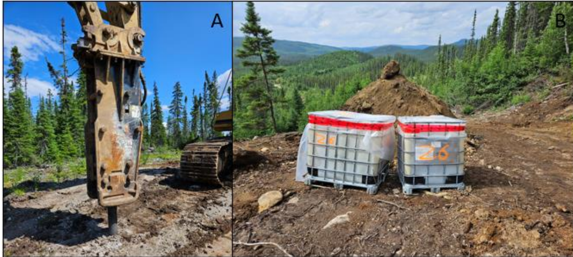
Figure 2: A) hydraulic hammer used to break the rocks; B) 1000L filled and sealed with painting indicating the zone from which the rocks are coming from
