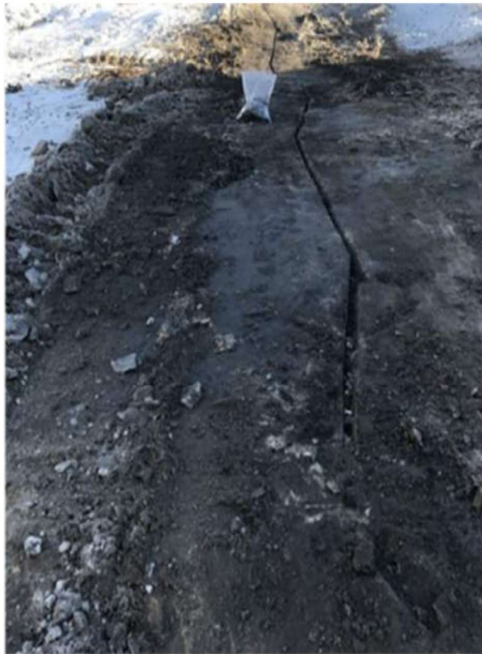
Zone 1: Channel sampling Graphite at surface 20% grade.
